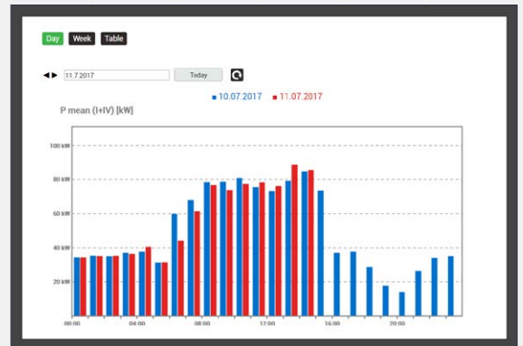
Current load profile of the day with values of the previous day via the device website
