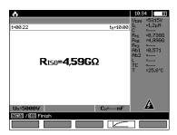
Both during and after measurement, the display can be switched back and forth between the results and the diagram by pressing **F4** ...
