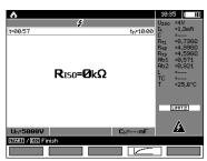
Even if puncturing occurs, the test instrument does not interrupt the measurement (as is the case with other measurements). The corresponding warning symbol appears at the top of the display.
