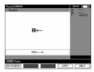
The test instrument is ready to perform a measurement. Use the **F4** LIMIT key in order to enter maximum resistance.
