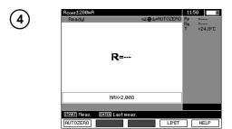
When AUTOZERO appears at the display, confirm that calibration of the measurement cables has been conducted. The test instrument is then switched to the measuring mode. AUTOZERO continues to appear at the display during measurement. Cable compensation remains active even after switching the test instrument off and then back on again.
