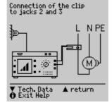
Alternating current can be measured in two measuring ranges (1 mA  $\dots$  10 A ~, 1 A  $\dots$  100 A~) with a clip-on current-voltage converter connected to the 2 and 3 jacks (e.g. the WZ12C).
