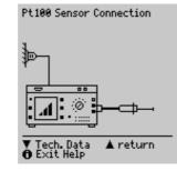
Temperature can be measured within a range of  $-200~^\circ\text{C}$  to  $+850~^\circ\text{C}$  with a Pt100 or Pt1000 sensor (default setting) connected to the PE (1) and N (2) jacks.
