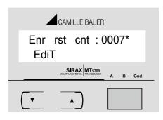
This screen enables user for setting maximum energy count after which energy will rollback to zero depends upon setting of Wh, kWh, & MWh. Pressing the " UP" key sets the displayed value and then SIRAX BT5700 exits from setup menu and starts normal operation. Pressing the "DOWN" key will enter the Energy digit reset count edit mode. This will scroll the value of reset count from 7 to 14 for Wh, from 7 to 12 for KWh & from 7 to 9 for MWh.
