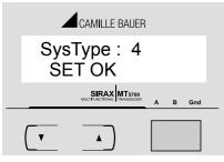
Pressing "UP" sets the displayed value and will advance to "Potential Transformer Primary Value Edit" menu. (See section 7.2.2) Pressing "DOWN" key will return to the system type "Edit" menu.
