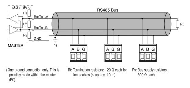
The signal wires (A, B) have to be twisted. GND (G) can be connected via a wire or via the cable screen. In disturbed environments shielded cables must be used. Supply resistors (Rs) have to be present in bus master (PC) interface. Stubs should be avoided when connecting the devices. A pure daisy chain network is ideal.
