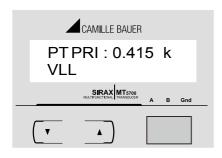
Pressing "DOWN" key enters into "Potential Transformer Primary Value Edit" mode. Initially the multiplier must be selected. Pressing the "DOWN" key will move the decimal point position to the right unit it reaches # # # .# after
