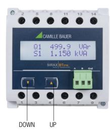
SIRAX BT5700 can be configured and programmed at site for the following: PT Primary, CT Primary, CT Secondary (5A or 1A) & three wire, three phase system or four wire, three phase system. The front panel has two push buttons through which the User may scroll through the available measurement readings, reset the energy (Import/Export) Min/ Max (System Voltage & System Current) & configure the product.
