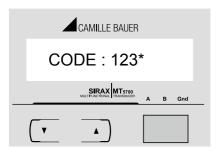
Enter Password, third digit entered, prompt for fourth digit. (\* Denotes that digit will be flashing). Use the "DOWN" key to scroll the value of the fourth digit from 0 through to 9, the value will wrap from 9 round to 0. Press the "UP" key to advance to verification of the password.
