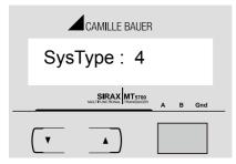
This screen is used to set the system type. System type "3" for 3 phase 3 wire & "4" for 3 phase 4 wire system. Pressing "UP" key accepts the present value and advances to the "Potential transformer Primary value edit menu 7.2.2 Pressing "DOWN" key will enter system type Edit mode and scroll between 3 and 4. Pressing "UP" key advances to the system type confirmation menu.
