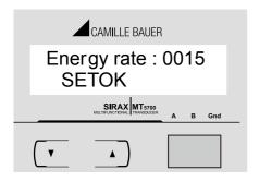
Pressing "DOWN" key re-enters into energy rate edit menu. Pressing "UP" key sets the displayed value as energy update rate and then advance the operation to Energy digit reset count menu (section 7.2.13). If energy rate is set to "00", then it sets "01" min as default value.
