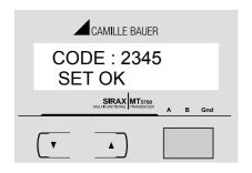
Pressing the "DOWN" key will return to the "New/Change Password". Pressing the "UP" key will advances to the system type Selection screen. (see section 7.2.1).
