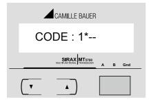
Enter Password, first digit entered, prompt for second digit. (\*Denotes that the digit will be flashing). Press "(DOWN) " key to scroll the value of the first digit From 0 through 9, the value will wrap from 9 round to 0. Press "UP" key to advance to next digit.
