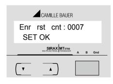
Pressing the " DOWN " key will re-enter Energy digit reset count edit mode. Pressing the " UP " key sets the displayed value and will exits from setup menu and starts normal operation.
