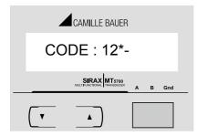
Enter Password, second digit entered, prompt for third digit. (\*Denotes that the digit will be flashing. Press " DOWN " key to scroll the value of the first digit From 0 through 9, the value will wrap from 9 round to 0. Press "UP " key to advance to next digit.
