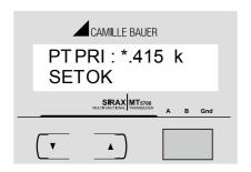
If scaling is to be corrected, pressing "DOWN" key will return to the "Potential Transformer Primary Value Edit" stage with the digits flashing indicating that the multiplier (decimal point position) should be selected. Pressing "UP" key sets the displayed value and then it will advance to Current transformer Primary Value selection menu (section 7.2.3).
