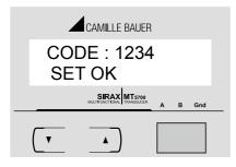
Pressing "DOWN" key will advance to the "New/change Password" entry stage (section 7.1.1)
