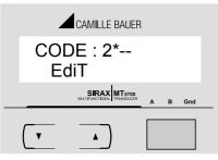
New / Change Password, first digit entered, prompting for second digit. (\* indicates that this digit will be flashing).
