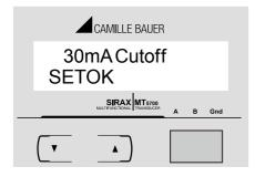
This screen allows user to set low start current cutoff at 30mA. Pressing "DOWN" key enters into edit mode and scrolls between Enable and disable. Pressing "UP" key accepts the selected option and enters Into 30mA cutoff confirmation screen.
