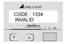
The unit has not accepted the Password entered. Pressing the "DOWN" key will return to the Enter Password stage. Pressing the "UP" key exits the Password menu & returns operation to the measurement reading mode.
