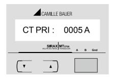
Pressing "DOWN" key will enter the "Current transformer Transformer Primary Value Edit" mode. This will scroll the value of the most significant digit from 0 through to 9, unless the presently displayed Current Transformer Primary Value together with the Potential Transformer Primary Value results in a maximum power of greater than 666MVA in which case the digit range will be restricted, the value will wrap.
