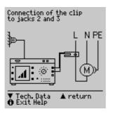
Alternating current can be measured in two measuring ranges (1 mA  $\dots$  10 A  $\sim$ , 1 A  $\dots$  100 A $\sim$ ) with a clip-on current-voltage converter connected to the 2 and 3 jacks (e.g. the WZ12C).
