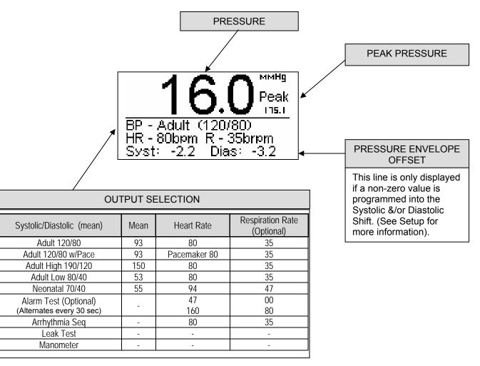
OUTPUT WAVEFORM SCREEN - This screen shows the pressure, peak pressure, output selection, and
